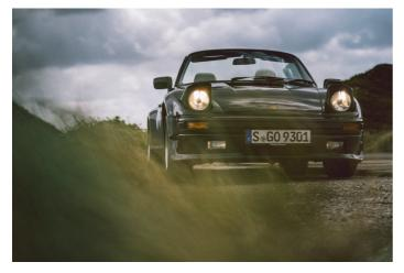
Like most Flatnose conversions, the car that I was supposed to drive for the following two days also received something called a 'power kit'. This adds an additional 30 PS over the normal 300, achieved thanks to a larger turbocharger, a quad-pipe exhaust system and an optimised charge-air cooler. All of which, of course, noticeably improves the performance and top speed.
