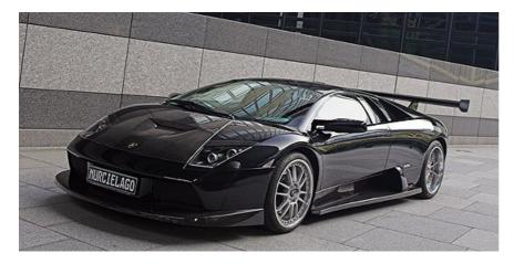
So the Murciélago receives an aggressive racing look like its FIA GT namesake, with a front spoiler/splitter, two-piece light alloy wheels, a large tail spoiler, transparent engine cover, plastic headlight covers, and louvred front bodywork.
